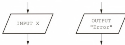
▲ Figure 7.7 Symbol used to show input and symbol used to show output
