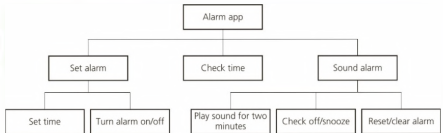
▲ Figure 7.3 Structure diagram for alarm app
