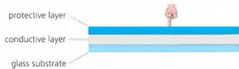
▲ Figure 3.32 Capacitive touch screen
