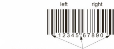
This shows the use of the guard bars separating the left from the right.
