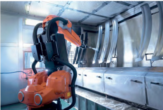
▲ Figure 6.18 Robot with spray gun end-effector
